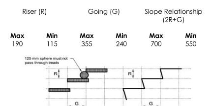
The risers and goings are to be constant throughout the flight and the stair treads must also have a non-slip finish or adequate non skid strip near the edge of the nosings.
